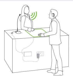
A Cross the Counter System is a hearing augmentation system that typically consists of a microphone and an amplifier / transmitter attached to a desk or small area. The amplifier transmits the speaker's voice or audio feed in a short range signal that can be picked up by a telecoil enabled hearing aid, cochlear implant (CI) processors, and specialized hand-held hearing loop receivers for individuals without telecoil compatible hearing aids.
